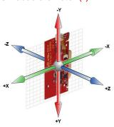
The module contains an optional 3D accelerometer (up to 16g), which can be used for a variety of custom specific (M2M) applications. Accelerometers are useful for measuring movement, speed, g-forces and vibration of the object. The accelerometer and advanced embedded firmware enables a very low-power battery solution.
